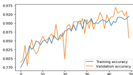
Figure 1. Accuracy of validation of the training process for VGG Net-16 for Tuta absoluta architecture. Blue line shows accuracy on training set, orange line shows accuracy on validation set.
