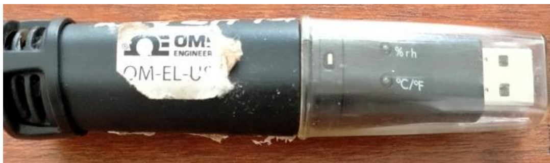
Figure 2. EasyLog USB electronic data logger device.
